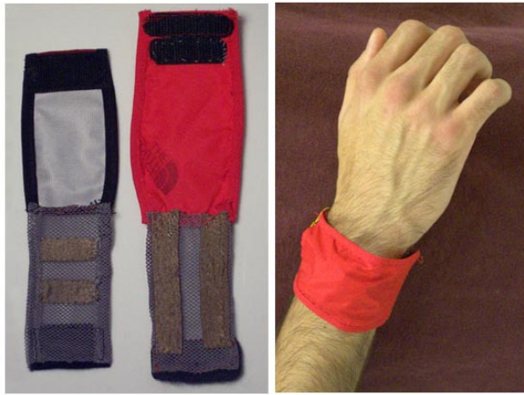
Fig. 2. Sensor band incorporating electrically conductive fabric electrodes.
