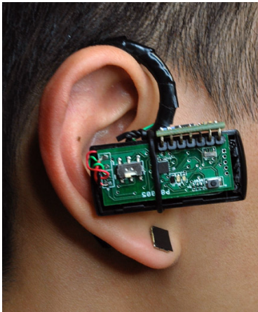
Fig. 4. Mobile photoplethysmography (PPG) sensor integrated into earring and wireless earpiece.
