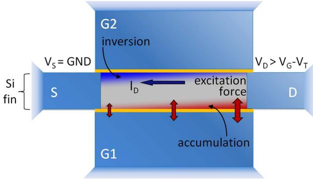
**Figure 2:** Top-view schematic showing principle of operation of a bulk-mode dielectrically transduced Resonant Body Transistor. The accumulation gate (G1) capacitively drives longitudinal waves in the fin while a FET channel generated by the inversion gate (G2) piezoresistively senses resonance.
