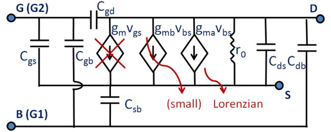
**Figure 3:** Small signal model of the RBT.  $g_m$  is the transistor transconductance through the front gate G2, and  $g_{mb}$  is that of back gate G1. Current due to the front gate is suppressed by DC biasing. The back gate effect is small, and defines the signal floor. The Lorentzian frequency response of the piezoresistive transconductance  $g_{ma}$  describes the high-Q electromechanical amplification at resonance.
