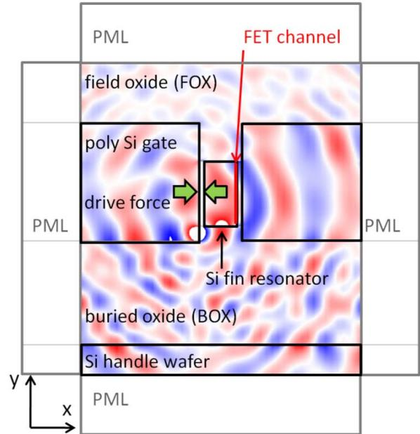
**Figure 4:** COMSOL simulation of side view of unreleased resonant mode in RBT, showing contour plot of stress along x-axis. A force applied across one dielectric (15 nm silicon nitride) generates a 1<sup>st</sup> harmonic longitudinal mode detected by strain induced in the FET channel. PMLs indicate regions of no reflected energy.
