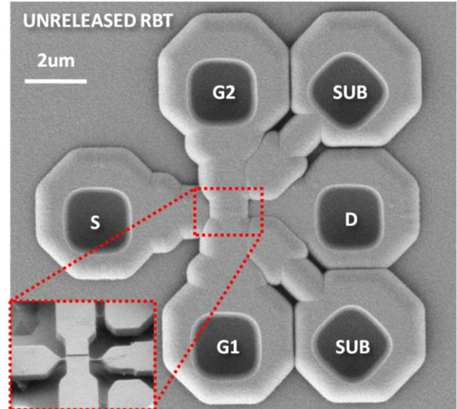
**Figure 1:** Scanning electron micrograph (SEM) of the unreleased RBT. The 1  $\mu\text{m}$  thick field oxide is visible on top of the unreleased resonator, showing contact holes to the silicon underneath. (Inset) Device with oxide cladding removed to show the underlying RBT.
