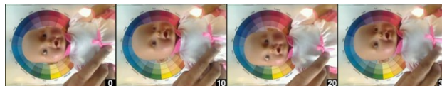
Figure 3. Video from a moving ambulance. The mannequin is being moved back and forth rapidly to simulate a seizure. Relative frame numbers are shown; the video is at 25 frames per second.
