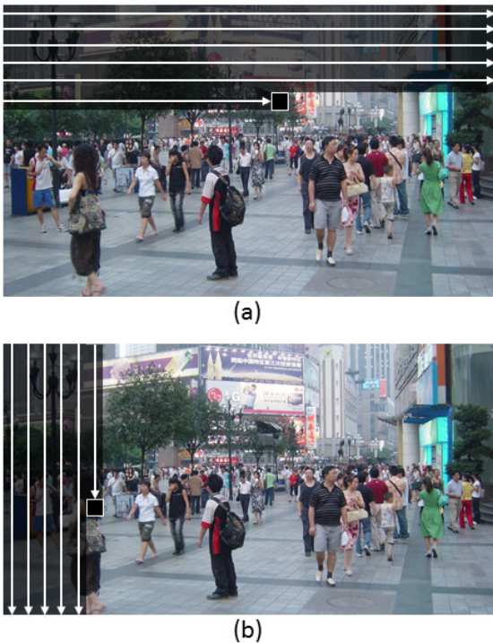
Fig. 5 Scanning order in reading the pixels from a frame (1080HD for this example). (a) Row raster scan. (b) Column raster scan.
