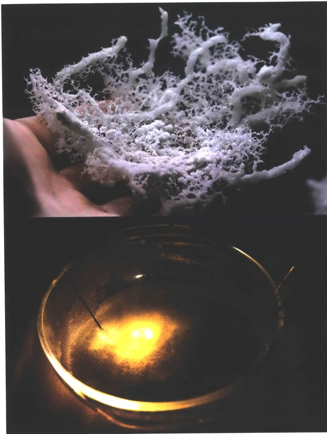
Figure 12: (A-bottom) Lichtenberg sintering electrode setup (B-top) Sintered glass Lichtenberg structure (Image credits: Steven Keating)
