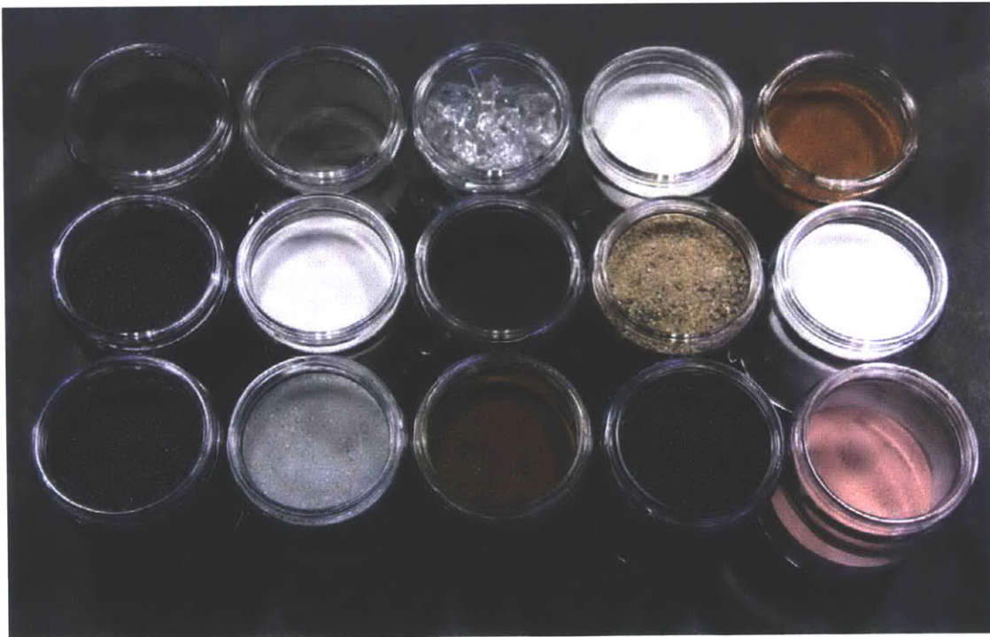
Figure 9: Varying glass compositions collected to experiment with additive sintering processes: Soda-lime glass #13-104 grits, recycled soda-lime glass, borosilicate, boromax frits, Moroccan sand, quikrete aggregate, black sand, magnetite sand, lunar and martian regolith
