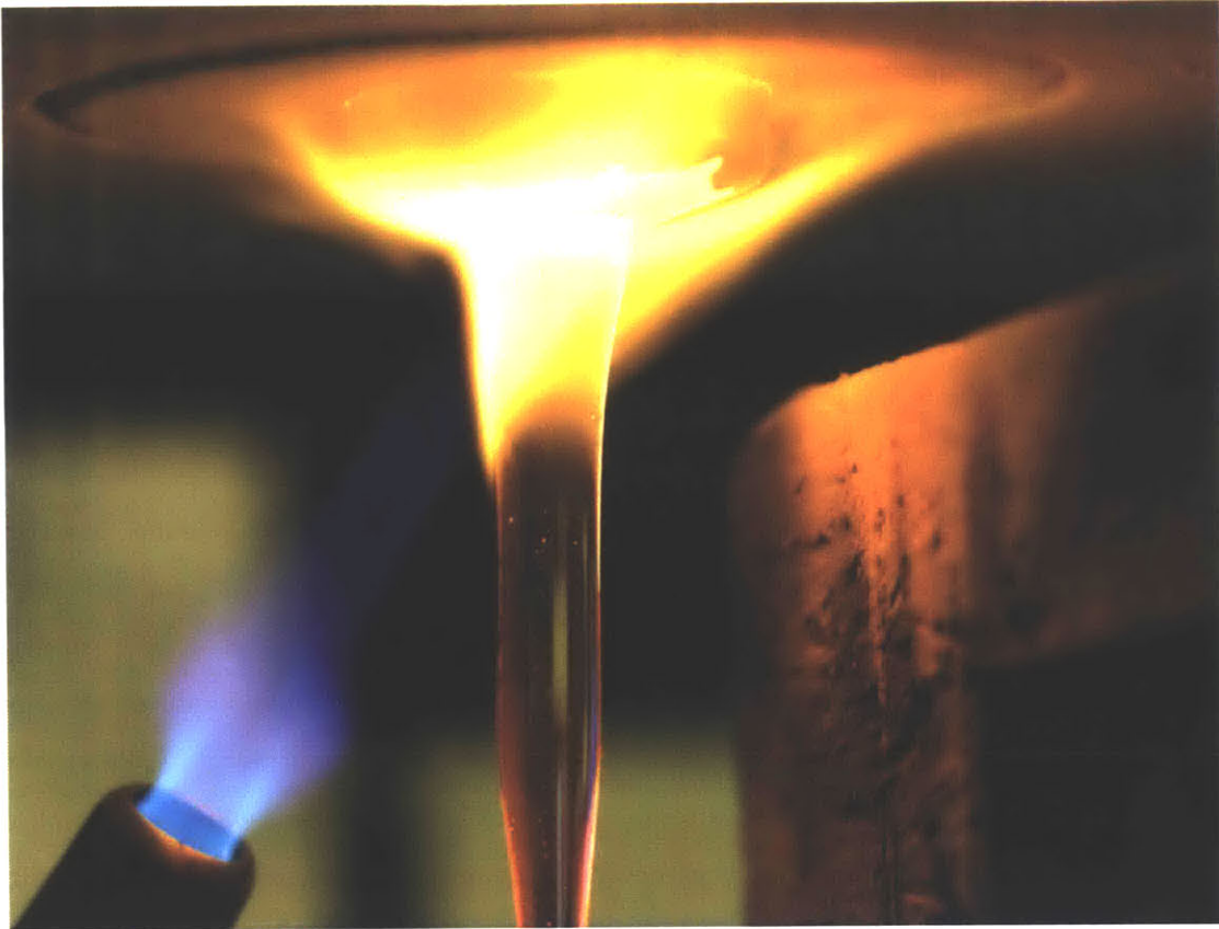
Figure 27: Molten glass flowing through the heated nozzle (Image credit: Steven Keating)
