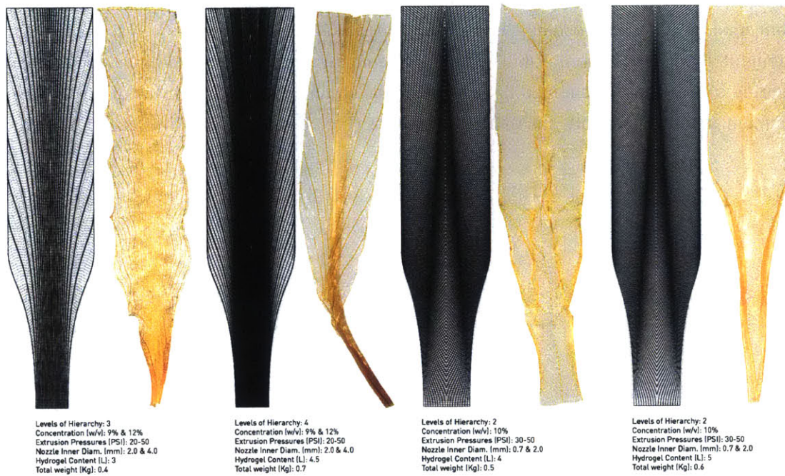
Figure 3-23: 2D tool path designs and their 3D fabricated counterparts using the HFP model.
