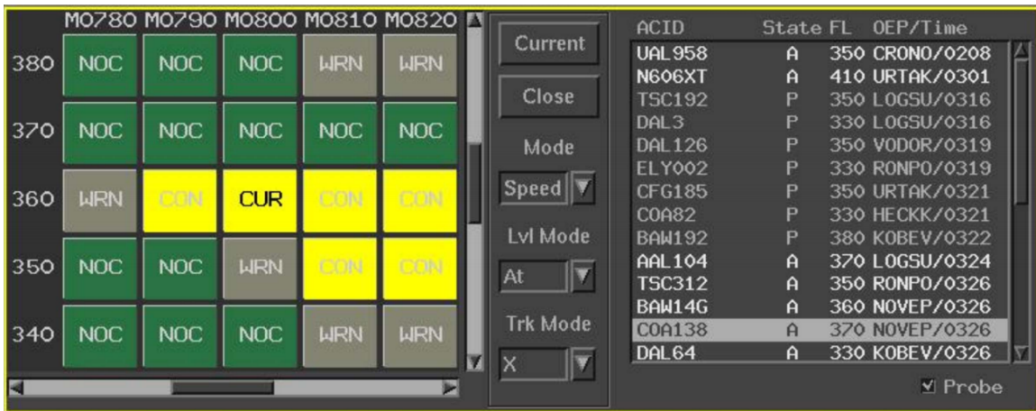
Figure 6: Bilateral Operations Resolution Grid (BORG) tool used for NAT assignment
