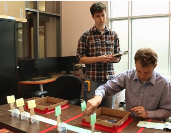
Fig. 3: This figure shows the participant verifying that one of the kits has all of the necessary parts and putting the parts one-by-one back into the part kit. This inspection is part of the fetching process. After verifying that the correct parts are located within the kit, the participant will bring the kit to the build stations. An experimenter is shown here instructing the subject on how to fetch a part kit before the experimental trials begin.
