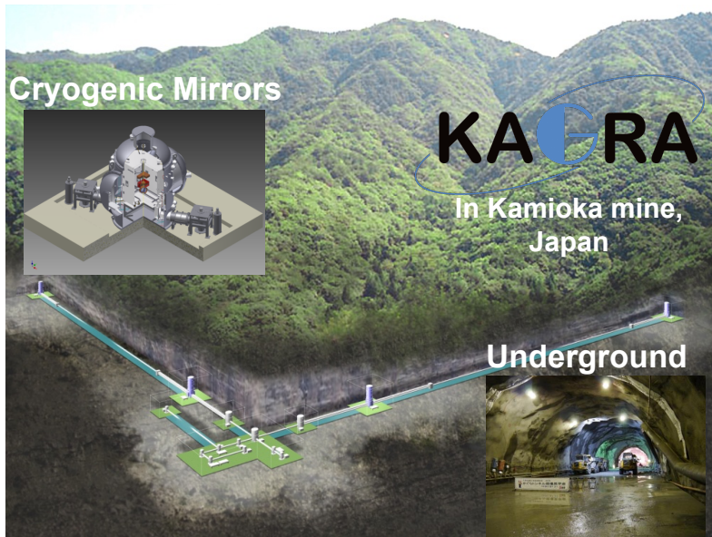
Fig. 6 Main features of the KAGRA detector: it is cryogenic, and built underground.
