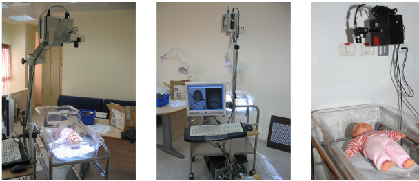
Fig. 13 Structured light scanner used to capture the facial geometry of newborns in the hospital.
