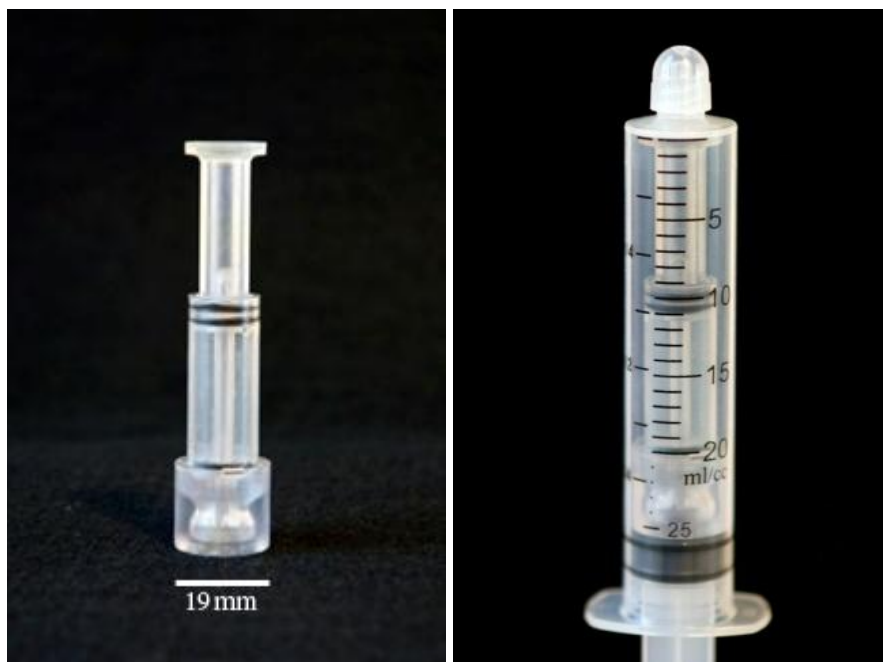
Figure 2: Fully assembled RRP device printed by 3D printer.
