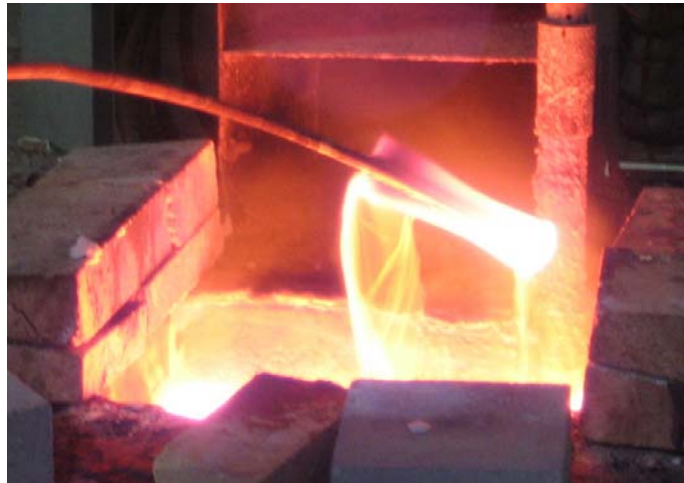
Fig. 5. Open air NaCl-KCl Salt bath at 900°C for metal heat treating. (Picture taken at Metallurgical Solutions, Inc in RI)
