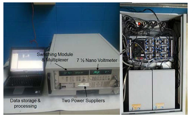
Fig. 3 Photograph of electronic components of ESAP-DCPD system
