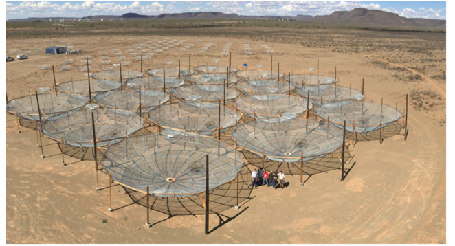
Figure 1. 19-element HERA layout used in this study, a subset of the full proposed 350-element layout. It is located in the South African Karoo Radio Astronomy Reserve. Each dish is 14 m across. The relative physical scale is illustrated by the group of people in this picture.
