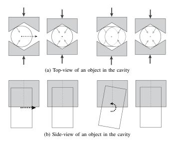
Fig. 3. Localization effect of V-groove cavity. Localization of a cylindrical object when offset in linear sense is shown on left, while that in angular sense is shown on right.
