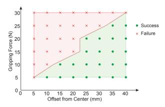
Fig. 6. Successful and failed pivoting experiments. The boundary between the regions is drawn for visualization purposes.
