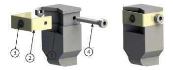
Fig. 1. Components of a two-phase finger: 1) V-groove cavity, 2) Elastic strip, 3) Point contact, and 4) Fastener. The assembled finger is shown on the right.
