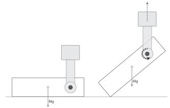
Fig. 4. Schematic of the pivoting phase. (left) The two-phase gripper holds an object offset from the center of gravity and (right) lifts it making it pivot about the fingertips. The bold arrow indicates the rotation of the object from the hand point of view.
