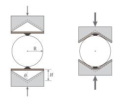
Fig. 2. Schematic of the change in contact geometry at the two-phase fingers as the grasping force switches from low (left) to high (right).
