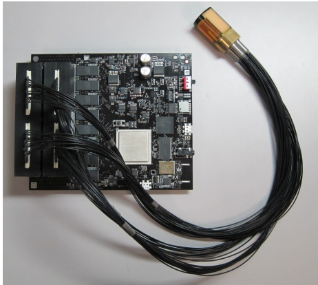
(a) Electrical hardware and custom transducer array.
