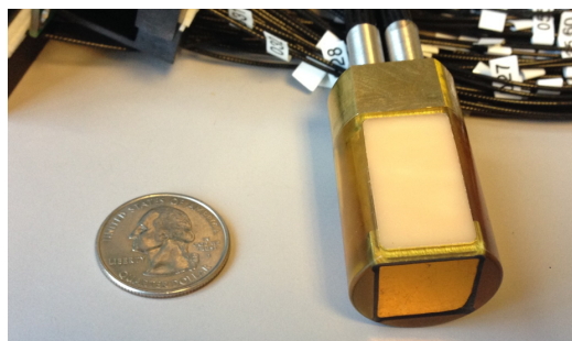
Figure 5-4: Custom two-dimensional transducer array for TCD instrumentation.
