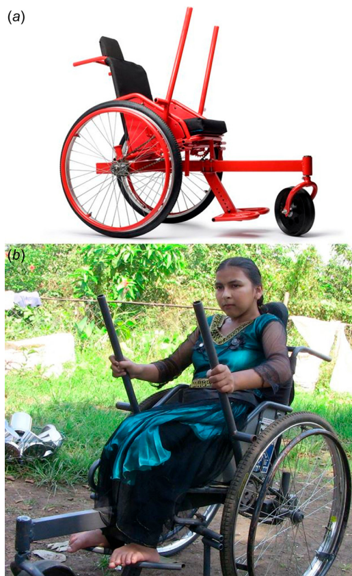
Fig. 1 The LFC. (a) Profile view of the LFC. (b) LFC user in India.
