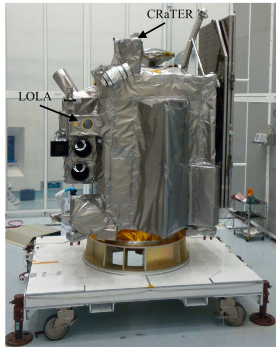
Figure 1. LRO spacecraft with the LOLA and CRaTER instruments identified. Image provided by X. Sun, NASA Goddard Space Flight Center. See Ramos-Izquierdo et al. [2009] for related images.
