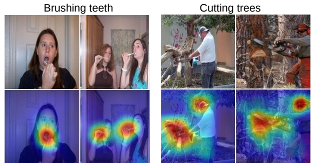
Figure 1. A simple modification of the global average pooling layer combined with our class activation mapping (CAM) technique allows the classification-trained CNN to both classify the image and localize class-specific image regions in a single forward-pass e.g., the toothbrush for brushing teeth and the chainsaw for cutting trees .
