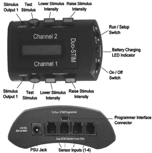
Figure 4 Duo-STIM system for drop foot [39]. Reproduced with permission from Elsevier.
