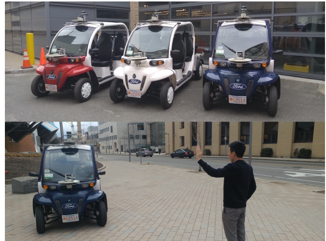
Fig. 1: A fleet of three electric shuttles operates on MIT campus. The shuttles are manually driven but equipped with camera and Lidar for sensing pedestrians. Customers may hail rides directly from any nearby shuttle.
