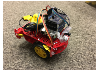
(b) UGVs are custom-build ground robots with onboard Raspberry Pi 2.
