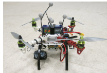
(a) UAV is a DJI F330 quadrotor with onboard Jetson TX1 flight controller.
