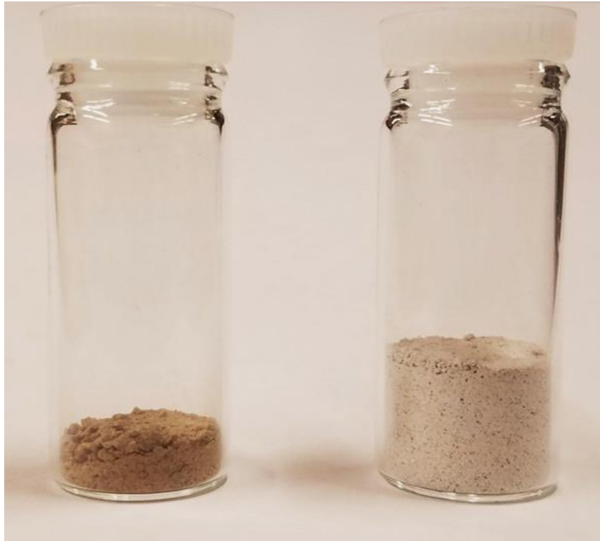
Figure ESI 3 Photographs illustrating the physical appearance of ultrapotassic syenite rock powder (left) and hydrothermal material (right). Both samples showed here are ~2 g. A much more loose packing and possibly a lower density are observed for the hydrothermal material rather than for the ultrapotassic syenite. Actual density measurements were not performed.
