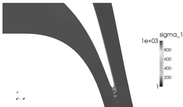
Fig. 8 Contour plot of divergence indicator \sigma_1 for the turbine vane, normalized by inverse of a single flow through time
