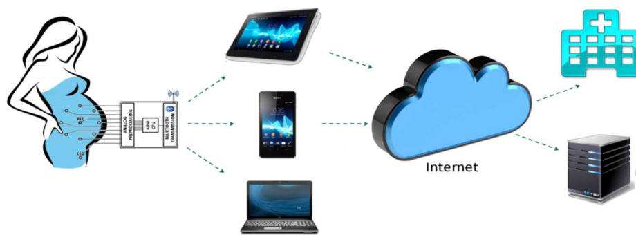
Figure 1. The Functional Diagram of the Telefetalcare System.
