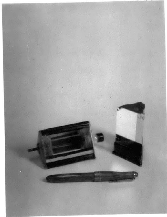
Fig. 9. WATER-FILLED AND GLASS PRISMS USED IN DUPLICATING NEWTON'S EXPERIMENTS. SCALE IS SHOWN BY FOUNTAIN PEN. LIQUID PRISM IS SEVENTH MODEL MADE, AND ONE ULTIMATELY USED SUCCESSFULLY.
