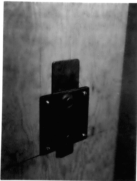
FIG. 10. ADJUSTABLE SLIT. APPROX 3" X 3". NOT CALIBRATED; SLIT-WIDTHS WERE MEASURED WITH GRADUATED RETICULE.
