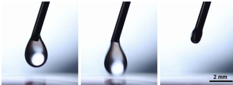
Figure S4. Time-lapse images of a droplet of pentane impinging on a flat copper surface; the contact angle is zero as the droplet completely spreads over the surface.
