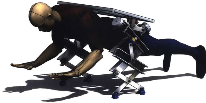
Figure 1-2: The Mantisbot Alpha concept with Supernumerary Robotic Limbs (SRLs). The SRLs support the upper half of the body and allow the worker to perform bi-manual tasks.
