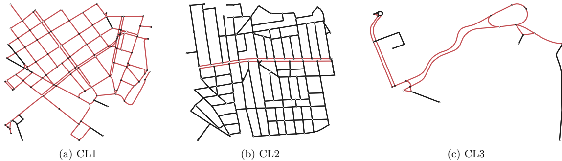
Figure 10: Sample of road network segments in São Paulo for clusters CL1 ( constrained ), CL2 - ( fine-grained ) and CL3 ( coarse-grained ) with c = 2.80, 1.82, 4.49 respectively.
