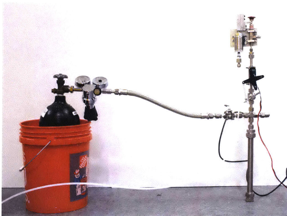
Figure 2-3: High temperature and pressure test apparatus used for validating the thermodynamics model presented here [25].
