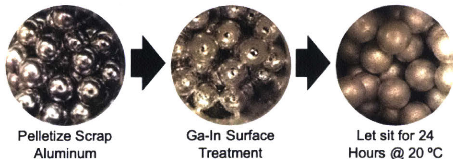
Figure 1-4: Basic process for converting scrap aluminum to a water-reactive fuel using a minimal gallium-indium surface treatment.
