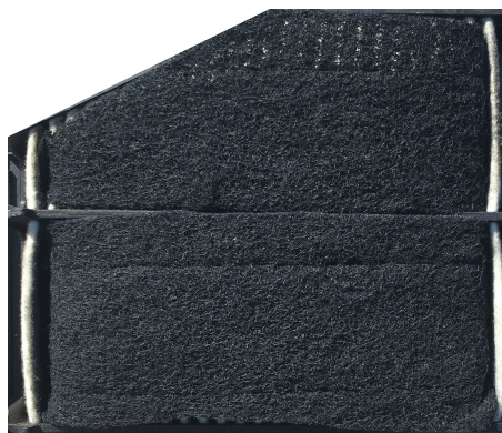
Figure 5: Simulation of filter loading using carbon filter material. Additional layers provide additional restriction, representing more significant occlusion.
