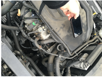
Figure 3: This photo shows the phone being moved across the engine's surface while recording audio. Relative motion is more representative of real-world use, e.g. when the algorithm is running self-contained as a mobile application.
