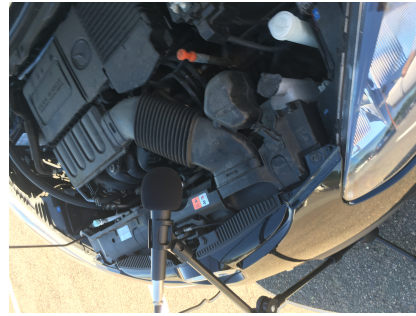
Figure 4: This figure shows a stand microphone placed over the air intake, to record flow data. The stationary microphone and proximity to the air intake minimized the impact of extraneous engine noise on the recording.
