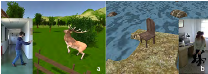
Fig. 13. User interactions in the virtual world. (a) Proximity based interaction with virtual elements (virtual world as seen from a first person perspective). (b) Interaction with a real chair through passive haptics (virtual world as seen from a third person perspective).
