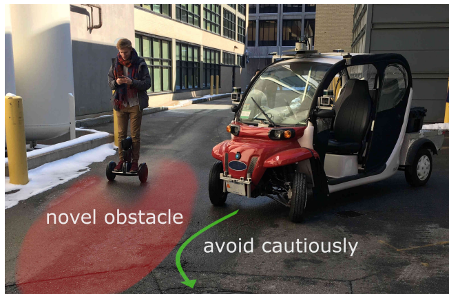
Fig. 1: An autonomous vehicle observes a novel dynamic obstacle that has never appeared during training, for example, an uncollaborative pedestrian on a personal vehicle. The proposed Reinforcement Learning framework detects the novelty and takes an action that cautiously avoids the pedestrian.
