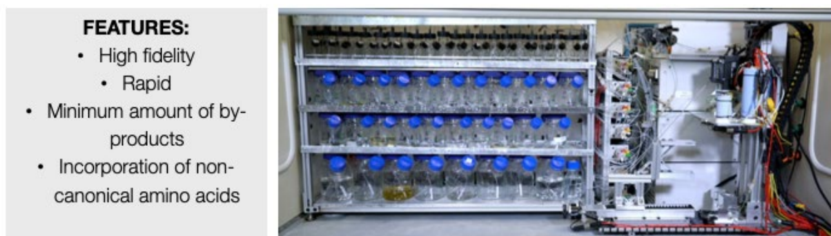
Fig. 1 Automated fast-flow solid-phase peptide synthesis enables high-fidelity production of long amino acid sequences. A) Fully automated chemical flow synthesis yields peptide chains, which —after purification and folding— give functional proteins; B) Automated fast-flow peptide synthesizer (AFPS) and main advantages of flow chemistry for solid phase peptide synthesis (SPPS).
