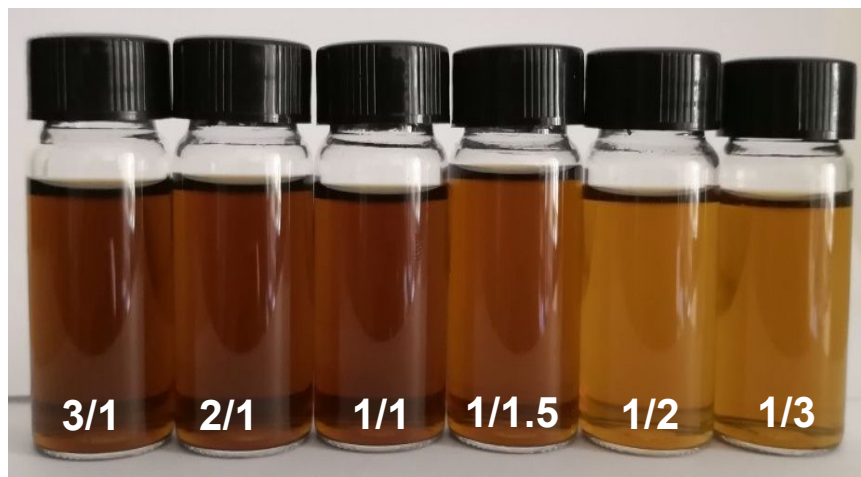
Figure S6. Photographs of N-doped CND samples prepared using the SPMA method with C/U weight ratios of 3/1, 2/1, 1/1, 1/1.5, 1/2, and 1/3, showing almost no sediments after six months.
