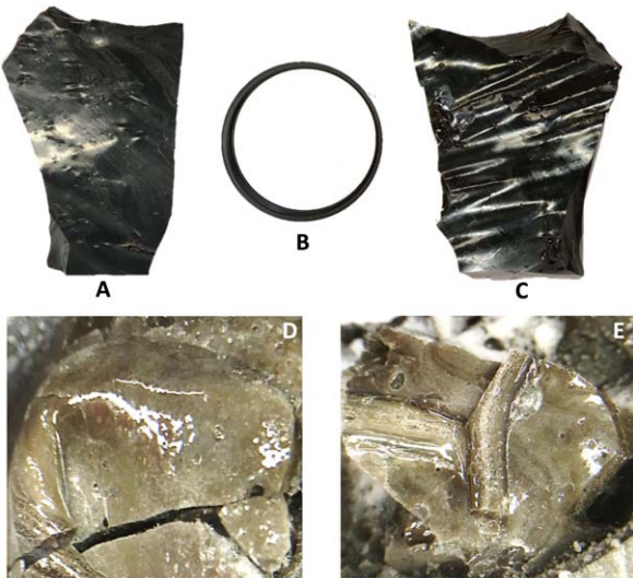
Figure 3. Quenched glass samples used to measure reflection. (A) Smooth basalt glass; (B) 99% white reflectance standard; (C) rough basalt glass; (D) smooth feldspar glass; (E) rough feldspar glass.
