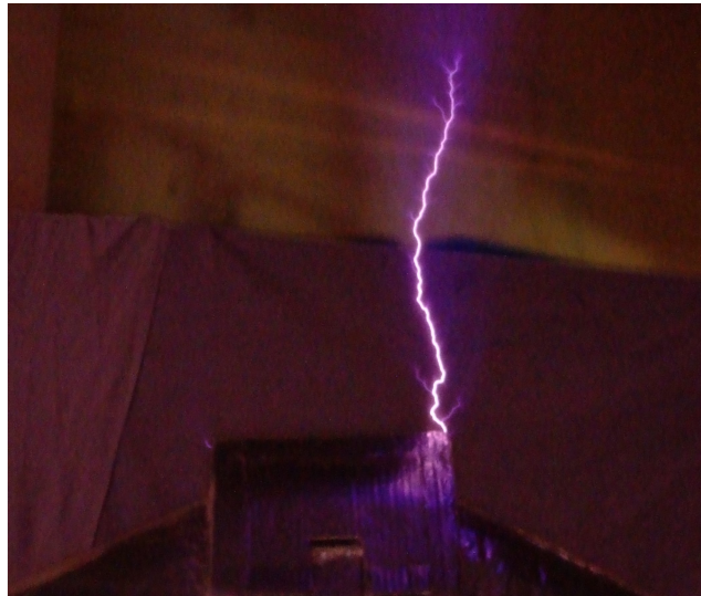
Figure 6. Representative photograph of aborted positive leader originating from model (3s camera exposure). The total length of this aborted leader, measured along the leader path and accounting for its tortuosity, is 44cm.
