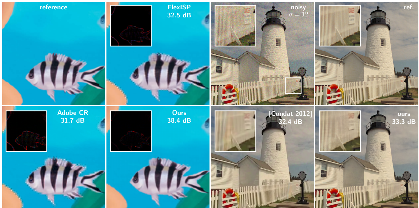
Figure 1: We propose a data-driven approach for jointly solving denoising and demosaicking. By carefully designing a dataset made of rare but challenging image features, we train a neural network that outperforms both the state-of-the-art and commercial solutions on demosaicking alone (group of images on the left, insets show error maps), and on joint denoising–demosaicking (on the right, insets show close-ups). The benefit of our method is most noticeable on difficult image structures that lead to moiré or zippering of the edges.
