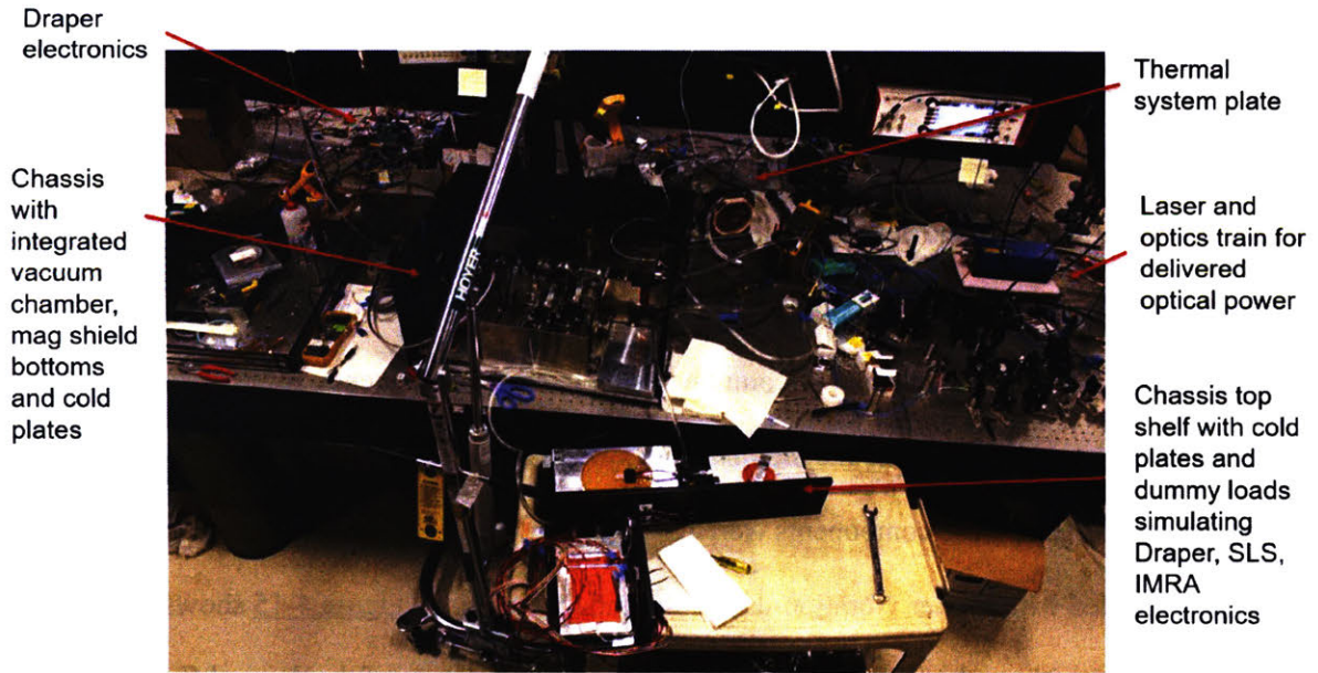
Figure 4-16. Frequency reference, chassis, and thermal control electronics integration at Draper.
