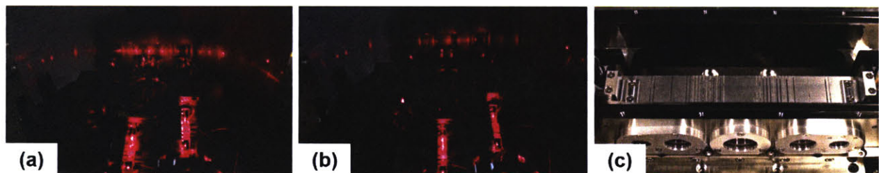
Figure 3-18. (a) Light scatter from optics without background mitigation; (b) light scatter from optics with three baffle cards placed in air-side locations; (c) blackening agent used inside vacuum chamber and also to coat the back surface of R-B optics in-vacuum to further reduce background light.
