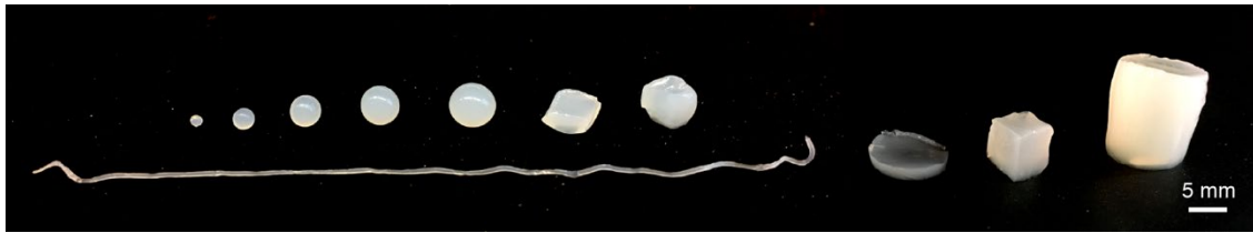
Supplementary Fig. 1 | Alginate cores in various geometries. The alginate core used to encapsulate cells can be shaped into spheres with different radii through extrusion with syringes and needles on parafilm followed by crosslinking in calcium chloride solution. Alginate thread was produced by direct extrusion in calcium chloride solution. Disk, cube, and cylinder-like structures can be achieved through cutting.
