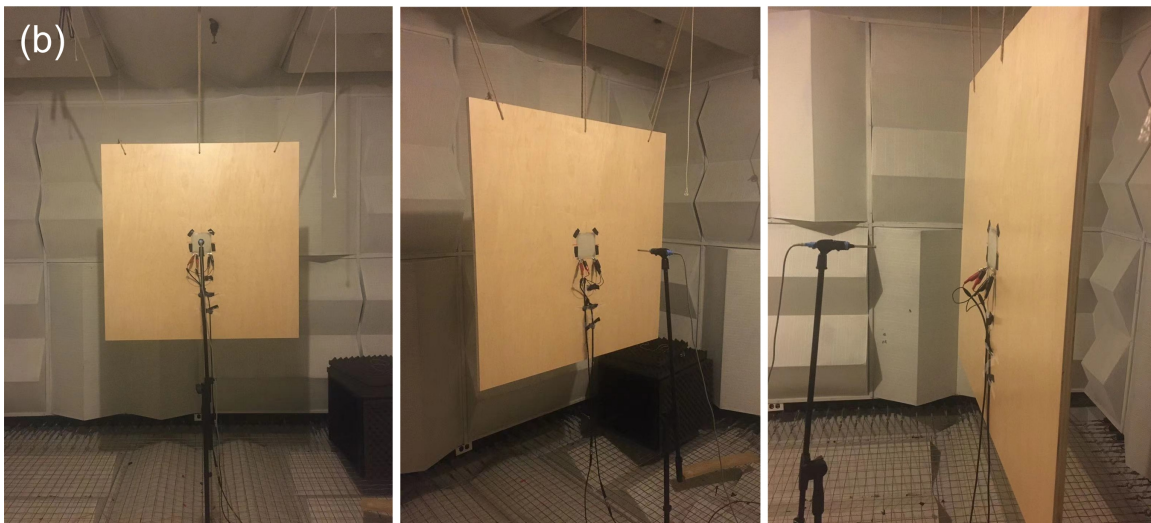
Figure 8-2: (a) Schematic and (b) pictures of the acoustic measurement setup in an anechoic chamber.
