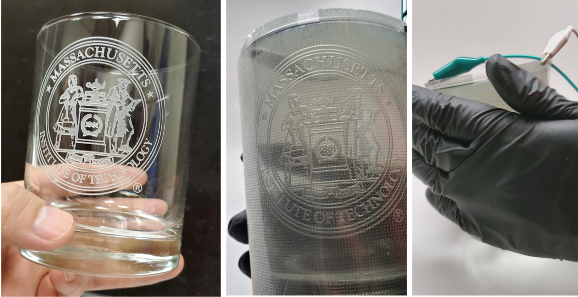
Figure 9-1: Pictures of a glass mug speaker enabled by a flexible, robust and transparent acoustic surface.
