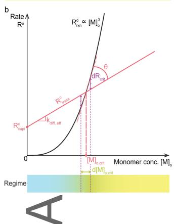
**Figure 2.** Relative rate dependence and resulting final composite morphology. (a) Definition of the different kinetics regimes based on the relative magnitudes of the transport rate and the reaction rate, as well as the expected resulting morphology. (b) Qualitative representation of the dependence of the different rates involved in ISIP on monomer concentration.
