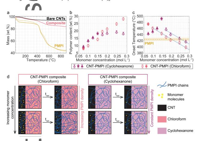
**Figure 5.** Thermogravimetric analysis (TGA) of the CNT-PMPI composites. (a) Representative TGA decomposition profiles obtained for the bare CNT structure, the pure polymer, and the composite. The solid and dashed yellow lines correspond to PMPI synthesized by IP in the absence of CNTs in chloroform and cyclohexanone, respectively. (b) Evolution of the polymer content in the composite with monomer concentration. (c) Evolution of the decomposition temperature of the PMPI in the
