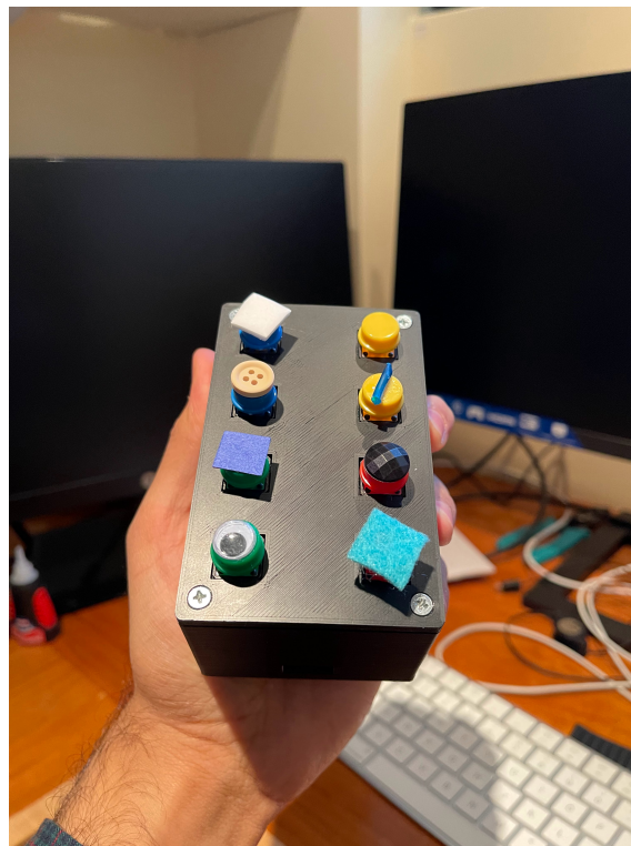
Figure 1-2: Device shown with physically distinguishable inputs.
