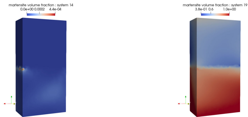
(i) Martensite volume fraction in system 14 at \epsilon = 2\% (j) Martensite volume fraction in system 19 at \epsilon = 2\%
