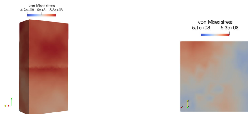
(a) Von Mises stress at a bi-crystal cross section parallel to x - z plane at \epsilon = 0.3\% (b) Von Mises stress at a bi-crystal cross section parallel to x - y plane at \epsilon = 0.3\%
