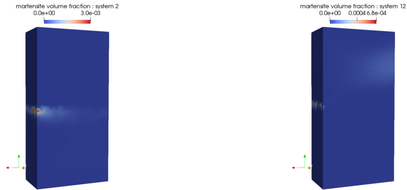
(g) Martensite volume fraction in system 2 at \epsilon = 2\% (h) Martensite volume fraction in system 12 at \epsilon = 2\%
