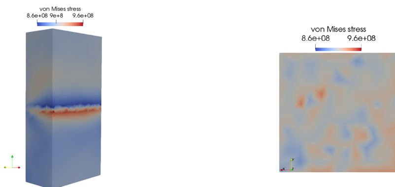
(a) Von Mises stress at a bi-crystal cross section plane parallel to x - z plane when \epsilon = 0.6\% (b) Von Mises stress at a bi-crystal cross section plane parallel to x - y plane when \epsilon = 0.6\%
