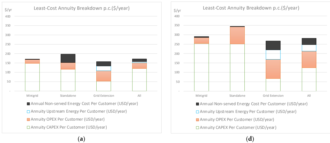
Figure 20. (a) Reference Scenario and (d) Double Demand Scenario cost of service breakdown including CAPEX, OPEX, Upstream Energy and CNSE.
