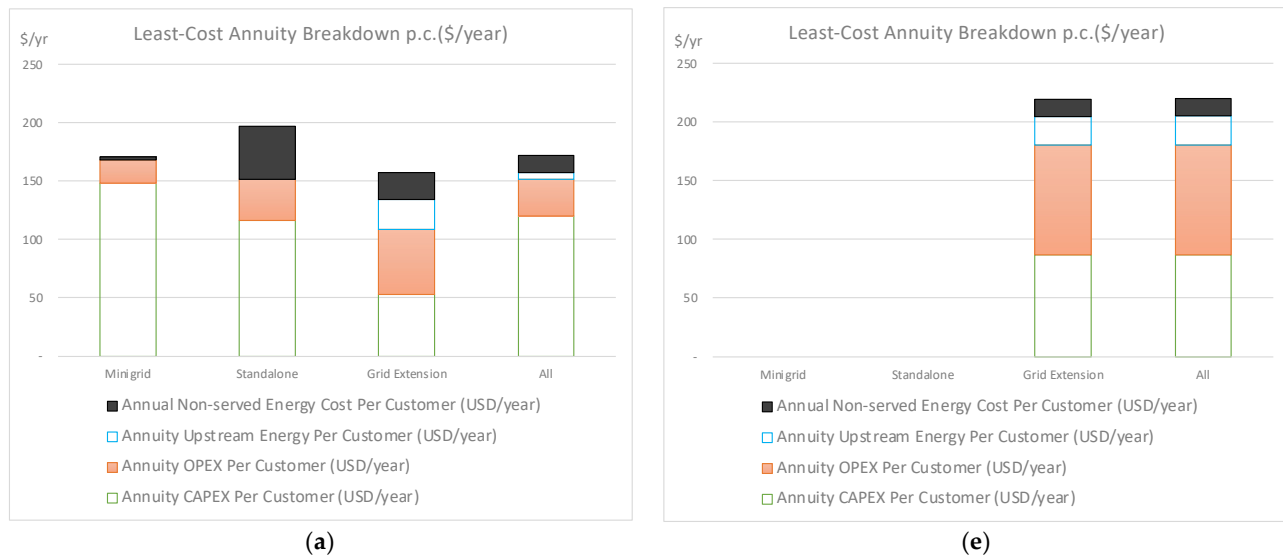
Figure 21. (a) Reference Scenario and (e) 100% Grid Extension Scenario cost of service breakdown including CAPEX, OPEX, Upstream Energy and CNSE.
