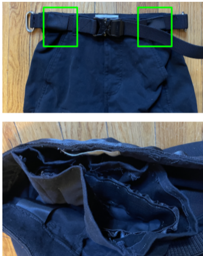
Figure 5-3: These images show the final prototype of the harness embedded pants. The vertical straps of the harness are secured to the front of the belt (highlighted in green). The bottom image shows the inner fabric layer with the two leg loops and respective elastics sewn into them.
