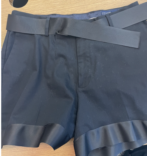
Figure 5-1: This image shows the first proof-of concept prototype. Note that the vertical straps connecting the leg loops to the belt are missing, and the bottom of the pants are also missing.
