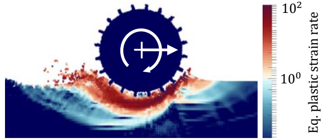
Figure 4-3: A sample high-speed rigid-wheel continuum simulations using MPM. The field being plotted is the equivalent plastic strain-rate.
