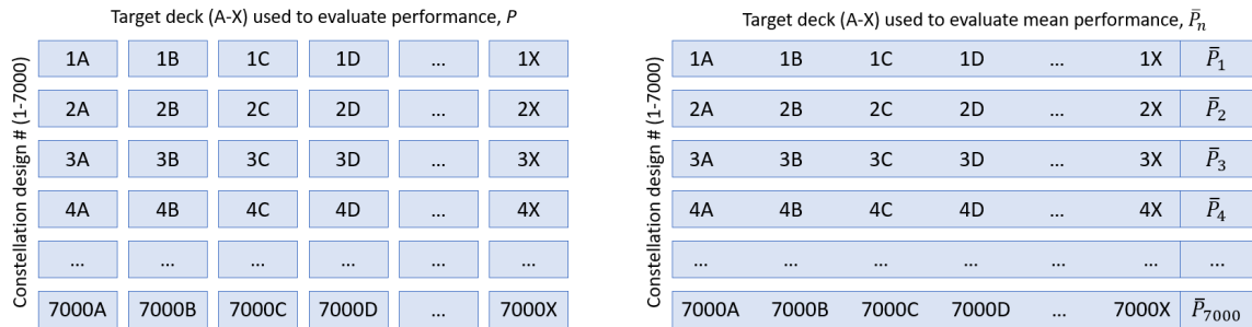
Figure 5-1: Visual comparison of code executions (left) consisting of one constellation design evaluated against one target deck, against functional evaluations (right) consisting of one constellation design evaluated against 24 target decks to arrive at an averaged performance value
