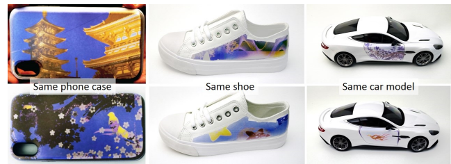
Figure 4: The same phone case and the same shoe re-programmed two times with different textures.
