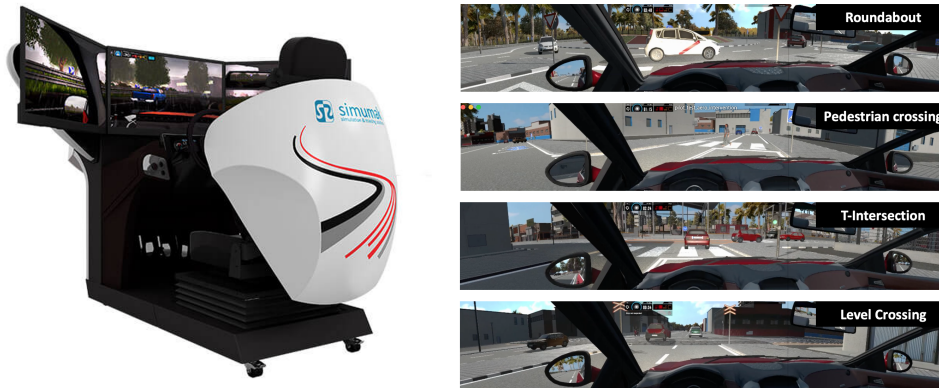
Fig. 1. The SIMUMAK car simulator and the sample images of simulated driving scenes
